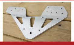
Redline Performance has developed strengthening drop brackets that do not require cutting of the tunnel or removal of your drop brackets. Simply slip our brackets over top of your stock ones and rivet / bolt in. Looks clean and strengthens your tunnel and drop brackets.
